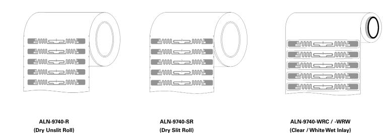
Standard Alien Inlay rolls unwind with metal antenna side facing outward, with respect to the core.
