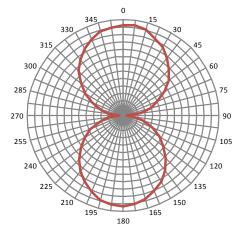
Angular Sensitivity (Relative Read Range vs. Orientation)
